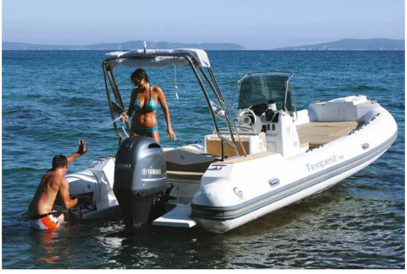
LENGTH O.A. 7,15 mt BEAM O.A. 2,85 mt TUBE DIAMETER 0,58 mt max DRY WEIGHT (approx.) 1050 kg MAX. PEOPLE ON BOARD 16 MAX. ENGINE POWER 225 HP (1 XL) CERTIFICATION CE С TUBE Neoprene - Hypalon Orca® 1670 dtex
