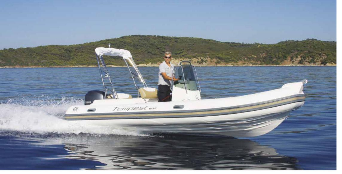
LENGTH O.A. 5,92 mt BEAM O.A. 2,50 mt TUBE DIAMETER 0,55 mt max DRY WEIGHT (approx.) 600 kg MAX. PEOPLE ON BOARD 12 MAX. ENGINE POWER 140 HP (1 L) CERTIFICATION CE Neoprene - Hypalon Orca® 1670 dtex TUBE
